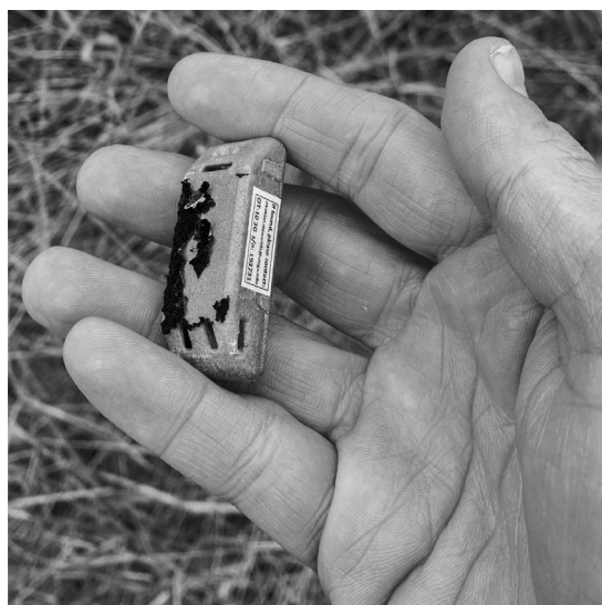
Figure 4. OrniTrack-10 GPS-GSM transmitter recovered from an adult female Gray Hawk 20 d after deployment; none of the Teflon harness material was found. We initially assumed the hawk had been killed because of the complete removal of the harness and most of the neoprene, but she was later resighted.
