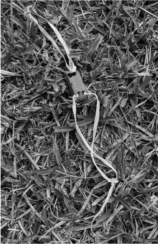
Figure 5. OrniTrack-10 GPS-GSM transmitter with what remained of the Y-transmitter Spectra harness, recovered from an adult female Gray Hawk. She removed the harness by biting through the sternum-connecting-ribbon in <27 d.
